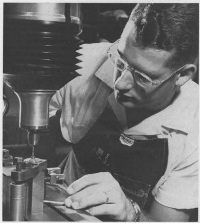
VERSATILE EXPERIENCE is gained in the Special Machine Section by apprentice Kyle Williams. Here he is using a jig grinder to shape the inside diameter of a tiny cylinder of alnico metal.
